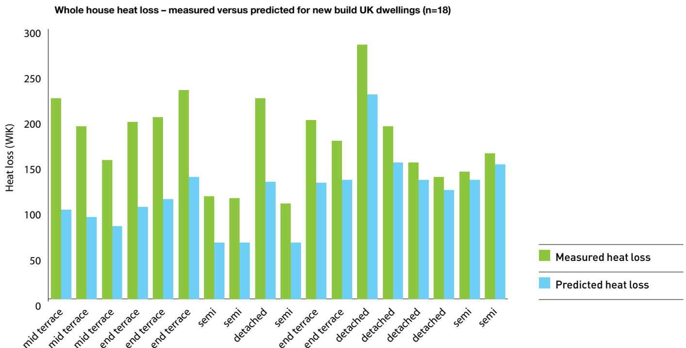
Fig.3a: Differences between predicted and measured whole house heat loss [Wingfield et. al., 2008], [Wingfield et. al., 2011], [Miles-Shenton et. al., in press, a], [Wingfield, Miles-Shenton and Bell, 2009], [Wingfield, Bell and Miles-Shenton, 2010]
